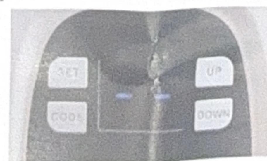
Press and hold the desired button on your Wireless Touch Wall Push Button that you would like to operate your door until the dots shown on the display flash.
