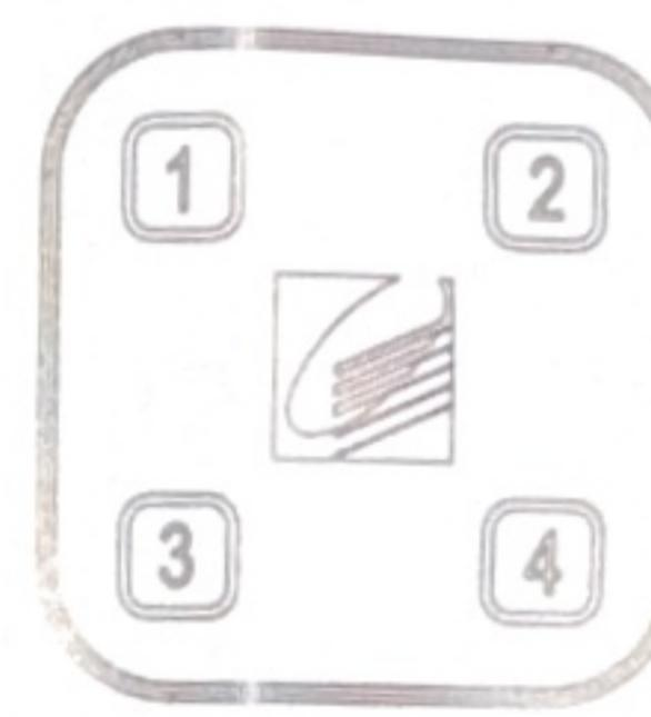
Press and hold your preferred button on the Wireless Touch Wall Push Button. The unit will beep twice to confirm successful coding. Wait approx 3 seconds for the unit to exit setup mode.
