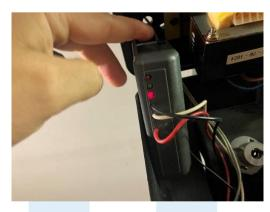
3. Open the small compartment on the left-hand side of the receiver as per the image below.
